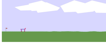
Figure 12: Halfcheetah2D problem: a cheetah robot must locomote as far as possible in the environment, which is characterized by limited variations in the slope of the terrain.
